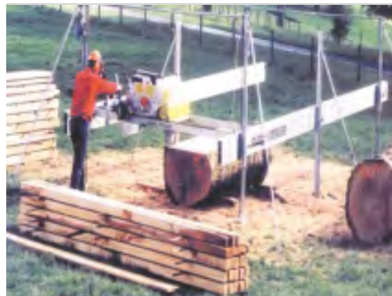
Plate 6. A portable circular saw which cuts horizontally on the forward run and vertically on the return. Forestor – Standrange Ltd
