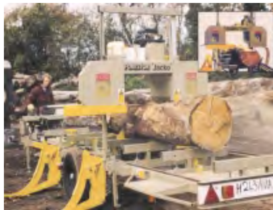
Plate 5. A mobile bandsaw making the first cuts through a log Forestor – Standrange Ltd
